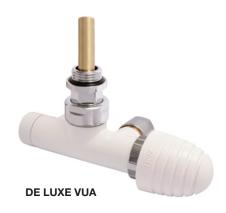
alternatively mirror-finished and chrome-plated, with screw cap, with single-bore connection to radiator. Radiator connection at bottom, thermostatic operation using HERZ DE LUXE Thermostat MINI, radiator can be taken off with pressurized system. Water flow control to radiator with single pipe operation: 40 %, pipe distance between centers: 50 mm.
