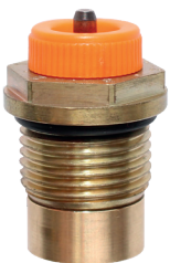
Thermostatic insert TS-98-V, 1 6367 98 (3/8", 1/2", 3/4") Protective cap orange Thread M 17 x 1.5 mm Presetting with key 1 6819 98
