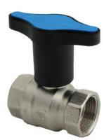
HERZ BALL VALVE MODEL 2201: models DN 15 (1/2") to DN 50 (2"), pressure class 25 bar; water, oil, recommended for heating systems. Handles in lever or wing shape, connections on both sides, internal thread in accordance with ISO 7, brass body nickel-plated, colour of handle red.
