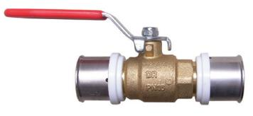
MODEL VARIANT PIPEFIX WITH PRESS CONNECTION FOR FLUSH MOUNTING (P72) for pipe dimensions 16 x 2.0, 20 x 2.0, 26 x 3.0, PN 10, water and sanitary installations, special bright brass.
