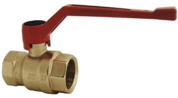
HERZ BALL VALVE MODEL 2211: models DN 15 (1/2") to DN 50 (2"), pressure class 25 bar; water, oil, recommended for heating systems. Handles in lever or wing shape, connections on both sides, internal thread in accordance with ISO 7, brass body nickel-plated, colour of handle red.
