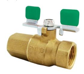
HERZ BALL VALVE MODEL (2304, 2305); Models DN 10 (3/8") to DN 50 (2"), pressure class PN 4 bar, for technical gases and gas installations in compliance with DIN DVGW G260, operating temperature -20°C to +60°C, steel handles in lever or wing shape, connections on both sides with internal thread or on one side with external thread in accordance with ISO 7, brass body nickel-plated, standard colour of handles yellow.
