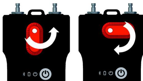
The connection of the pressure inlets can also be used to bleed the connection hoses of the measuring unit. For media temperatures above 50 ° C, venting of less than 10 seconds is recommended to avoid unnecessary heating of the pressure unit measuring circuits.
