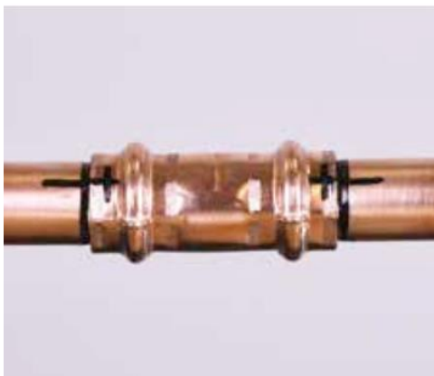
6. Mark the completed joint
