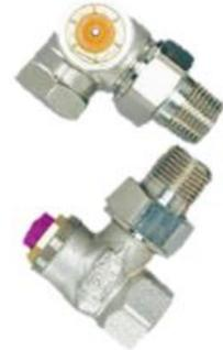
Pre-settable TRVs utilised in HIU space heating circuits, will ensure that radiators will receive correct design flowrates. This will, therefore maintain the temperature differential in the secondary and avoid the high primary return temperatures which can be caused by unbalanced space heating circuits.
