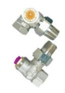
Presettable TRVs utililised in HIU space heating circuits, will ensure that radiators will receive correct design flowrates. This will, therefore maintain the temperature differential in the secondary and avoid the high primary return temperatures which can be caused by unbalanced space heating circuits.
