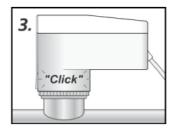
Simply latch the actuator to the valve adapter manually by applying vertical pressure; a clicking sound can be heard. Switch on the power suppy in the connection.
