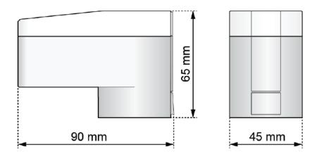
HERZ Motor Valve Drive, 3-point, M28 x 1.5, 230 V, 50 Hz normally closed, actuating force 200 N, operating voltage 230 V  $\sim$ , threaded connection M28 x 1.5, blue adapter 1 7708 85 is included, max. stroke 8,5 mm
