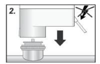
Position the actuator in deenergized state manually in vertical position to the valve adapter.
