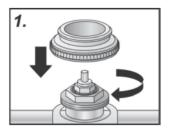
Screw the valve adapter manually onto the valve.
