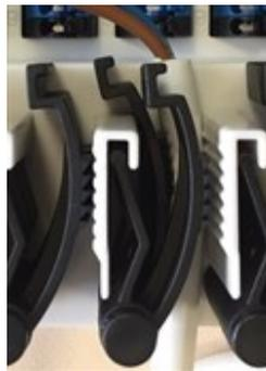
The strain reliefs are suitable for flexible cables with a cable sheath diameter of 5 mm to 8 mm, primarily using the lower strain relief (as shown). The cables must be checked for firm placement. Solid, thicker and thinner cables must always be laid firmly and must be fixed on the installation side.
