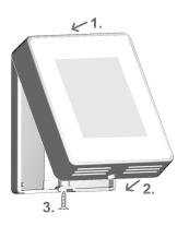
Open the connection terminals with the accompanying operating tool and make the electrical connection (24 VDC, GND, CAN-High and CAN-Low) as described in the operating manual of the Control Box.
