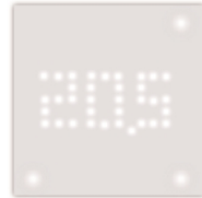
Measuring unit and measured value display The first touch of the touch area shows the temperature. Repeated touching changes to other measured values and first shows the unit and after a short time the measured value.
