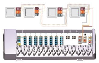
The 1-Wire system must be realised with 3 wires (5 VDC, DQ, GND). The wiring must be done in series, see diagram opposite. Stub lines should be avoided or made as short as possible. The total cable length can be up to 100 m. A suitable twisted pair cable must be used and sufficient conductor cross-section must be ensured, e.g. LIYCY 2 x 2 x 0.75 mm<sup>2</sup>, in order to avoid impermissible voltage drop at the HERZ clever&smart room sensors.
