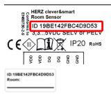
Each HERZ clever&smart Room Sensor has a unique 16-digit 1-Wire ID. This ID is required for sensor-room assignment in HERZ clever&smart Room Controller. The ID can be found inside the sensor on the type plate and on the supplied sticker. We recommend sticking the sticker in the table of the HERZ clever&smart Control Box instruction manual or in the HERZ clever&smart Control Box terminal plan sticker to simplify the later configuration of the system.
