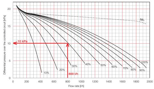
With a pre-setting of 40 % on the DN 20 LP 4012, valve 10 kPa of differential pressure will remain available to the circuit. The control valves within the circuit need to be sized such that they provide the required flow at this differential pressure (adjusted for pressure losses on piping and fittings). This means that an appropriate kv-value needs to be set at each the control valves:
