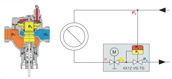
The HERZ 4012 VS-TS is constructed as a combination of a differential pressure regulating valve and a pre-settable control valve.
