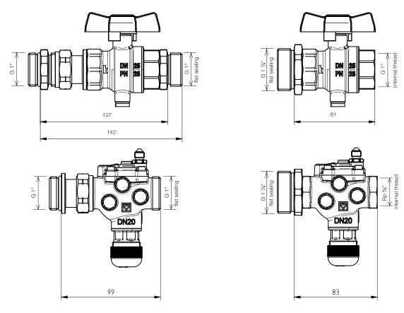
☑ Dynamic Regulation Sets for Underfloor Heating Manifolds
