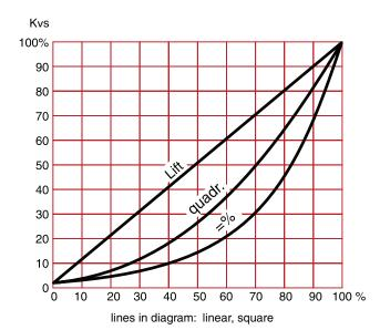
Linear valve characteristic could be changed by using the valve drive 1 7712 11 with fitted DIP switches.
