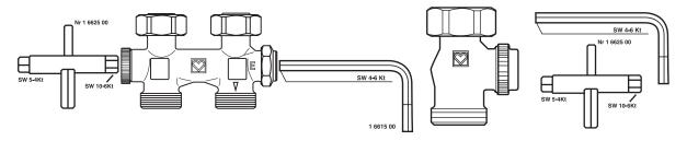
Fill and drain adapter, 1 0256 01, with hose connection, 1 6206 01, unscrew on the "E" side of the bypass body and place a vessel under the end.
