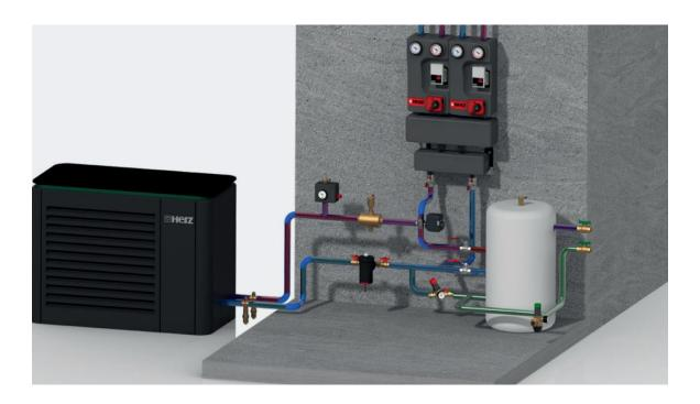
The integrated ball valve allows seamless isolation of the filling valve, while the check valve prevents mixing of heating water and potable water. This enhances both convenience and safety. By combining three essential functions—pressure reduction, isolation and backflow prevention—into a single unit, the HERZ Automatic Filling Valve also simplifies installation and increases system reliability.
