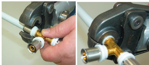
Complete pressure sealing using a press device or manual press pliers. The pipes must be free of stress. The press procedure is complete if the jaws have been closed completely.
