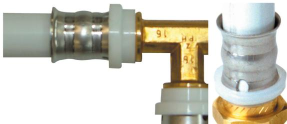
Checking the pressure sealing: On the side of the press sleeves you can see two parallel, ring-shaped grooves with a bulge between them.
