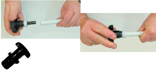
Placing the fitting on the pipe. Check the correct pipe engagement through the vision ports on the press sleeve - the pipe must have fully engaged on the fitting and be visible in the ports.
