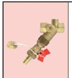
**ERZ Strainer** with draining valve, fine-mesh strainer chromium-nickel steel, body of dezincification-resistant brass - socket x socket.
