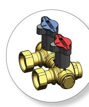
▶ HERZ multifunction ball valve block with red and blue handle, ball with T-bore. T-bore of the ball with full passage allows draining or filling of complete system or a partial system in case of maintenance. The position of the ball valves is indicated by the ball valve handles.
