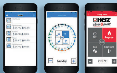
HERZ clever&smart app with display of individual rooms, individual setting of cooling/heating time and operating mode.
