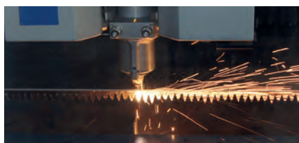
Modern laser system for processing structural steel, stainless steel and aluminum at HERZ Energietechnik in Pinkafeld.
