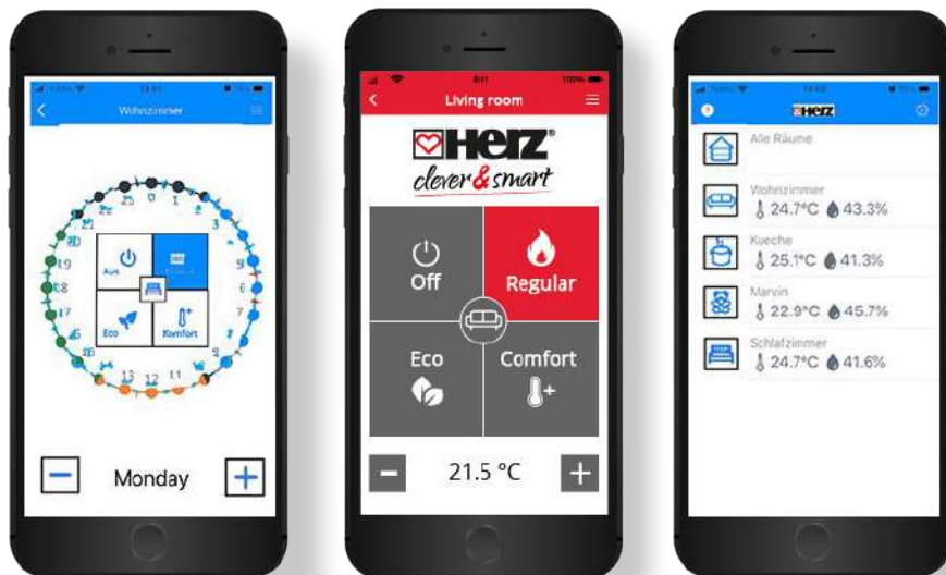
HERZ clever&smart App with display of the individual rooms, individual setting of the cooling/heating time and module selection.
